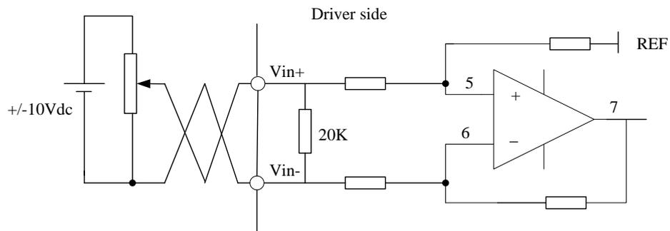
Figure 3-7 Analog Input Interface
