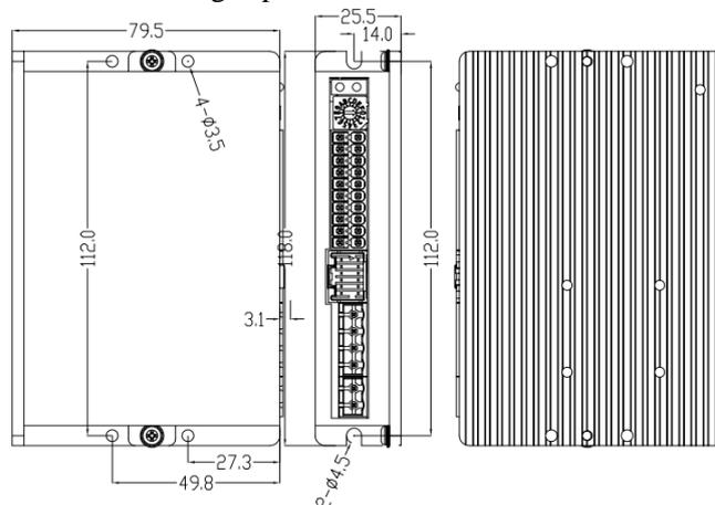
**Figure 2.1(A) installation method of drive ELD2-RS7005/ ELD2-RS7010**
