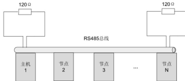
The correct connection of terminal resistance is shown in the above figure, a 120 ohm terminal resistance need to connect in the head end and the end of the communication bus.
