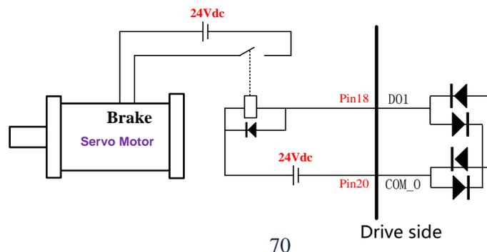
About the wire of brake, there should be an 24VDC for brake, the brake will be released with the 24VDC input, and the drive provide an output signal to control the connection or disconnection of the 24VDC, and it is forbidden to connect these signal directly for the power of 24VDC, it will destroy the hardware of servo drive.
