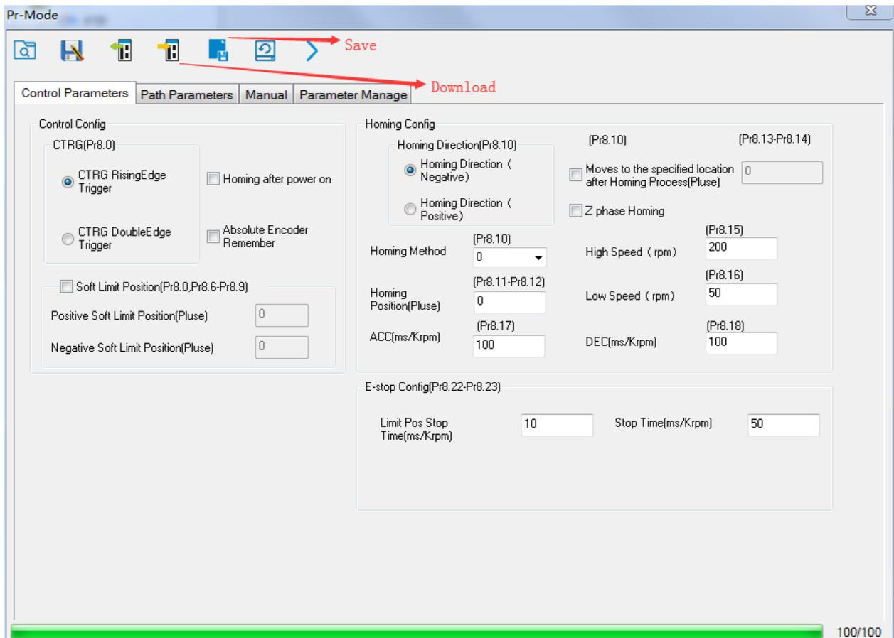
**Notes:** After the control parameter setting is completed, click the Download button of the toolbar to make the parameters valid. Click Save button to save the parameter to drive permanently.
