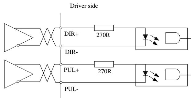
Figure 3-4 Pulse Input Interface Differential Drive Mode
