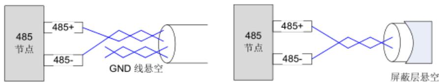
Firstly, confirm that the signal line of RS485 is connected correctly. Secondly, confirm whether the communication reference ground is connected correctly. If the node has no communication reference ground, it will be suspended, as shown in figure above. The shielding is connected the same way.
