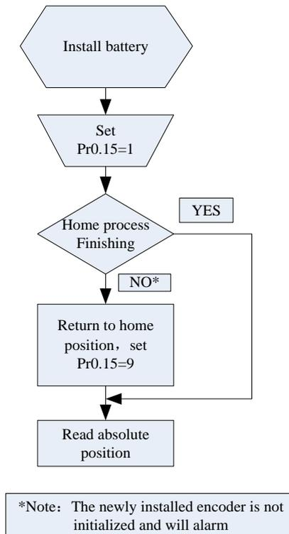
1) Firstly, select the motor with multi-turns absolute encoder which includes battery, and confirm if the drive version supports the function about multi-turns absolute encoder;
