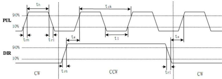
Figure 3.6 pulse + direction input interface timing (the maximum of pulse frequency : 500KHZ)
