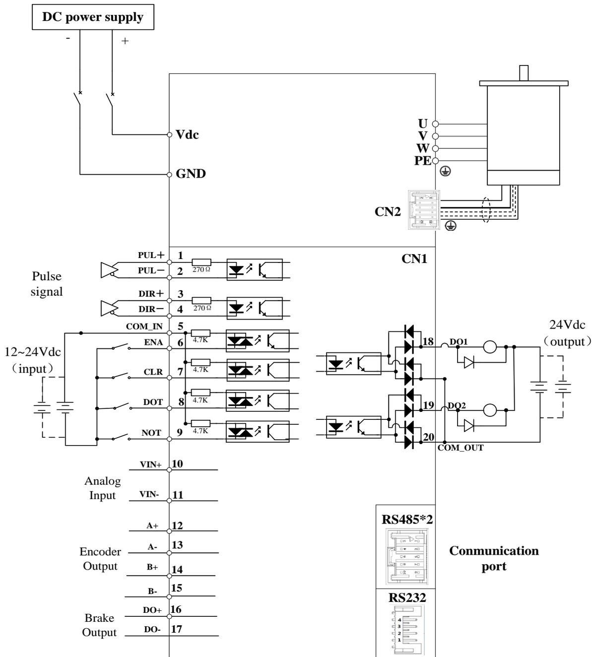
Figure 3-1 Position Mode Wiring
