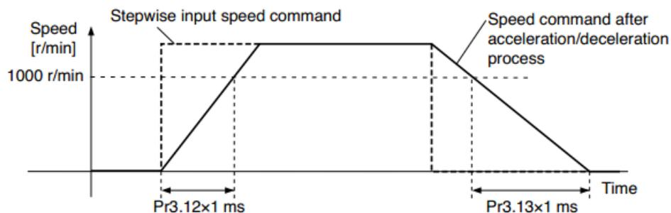
$$\text{Deceleration time (ms)} = V_c / 1000 * \text{Pr3.13} * 1\text{ms}$$
