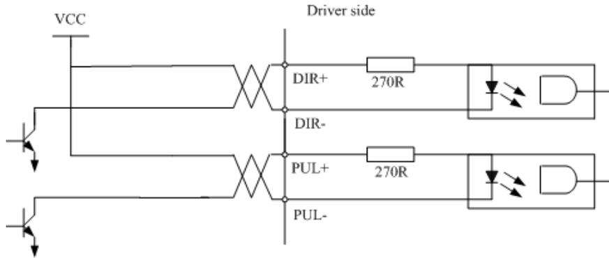
**Figure3-5 Pulse Input Interface Single Terminal Drive Mode**
