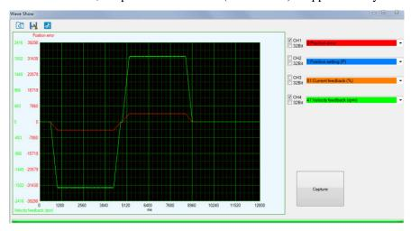
3. When keep decreasing the value pf Pr0.03, the position loop gain Kp become bigger and bigger, the integration time constant Vi become smaller and smaller, the position error becomes close to zero. When Pr0.03=62, the position error value (curve in red) is approximately 2000.
