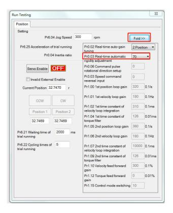
2. Click button "Servo Enable", then you can run the motor.
