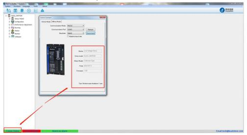
If the connection fails, make sure all cables are properly connected, the device is powered on and that you have selected the correct device and set the appropriate communication parameters.
