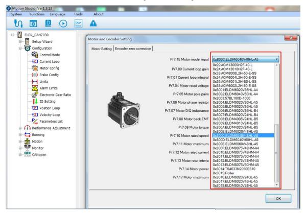
3. Select a matching motor model, press the button "OK", Complete the motor parameters setting.
