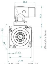
Power connector 4+4 PIN M23 turnable BEDC 110 - Signal connector 17 PIN M23 turnable AEDC 139
