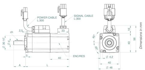
Power connector 6 PIN AMP 172168 - Signal connector 15 PIN AMP 172171
