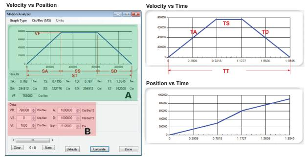
A Motion analyzer plot contains the graph, which may be viewed as velocity over position, velocity over time, or position over time, and a detailed analysis of the move.
