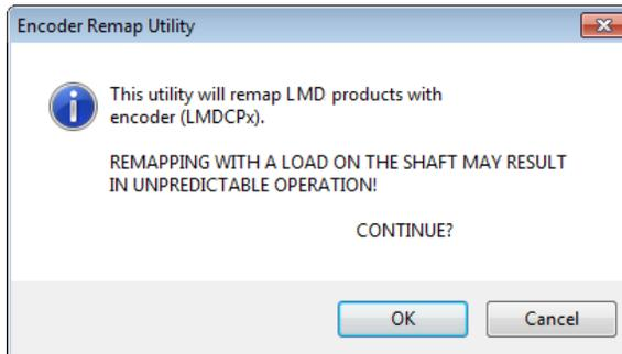
4. Verify motor shaft uncoupled from loads and free to move. Once communications is verified, acknowledge the understanding the motion will occur by clicking OK. The motor will turn one revolution clockwise, then one revolution counter-clockwise.
