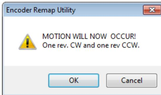
5. The motor will turn one revolution clockwise, then one revolution counter-clockwise.
