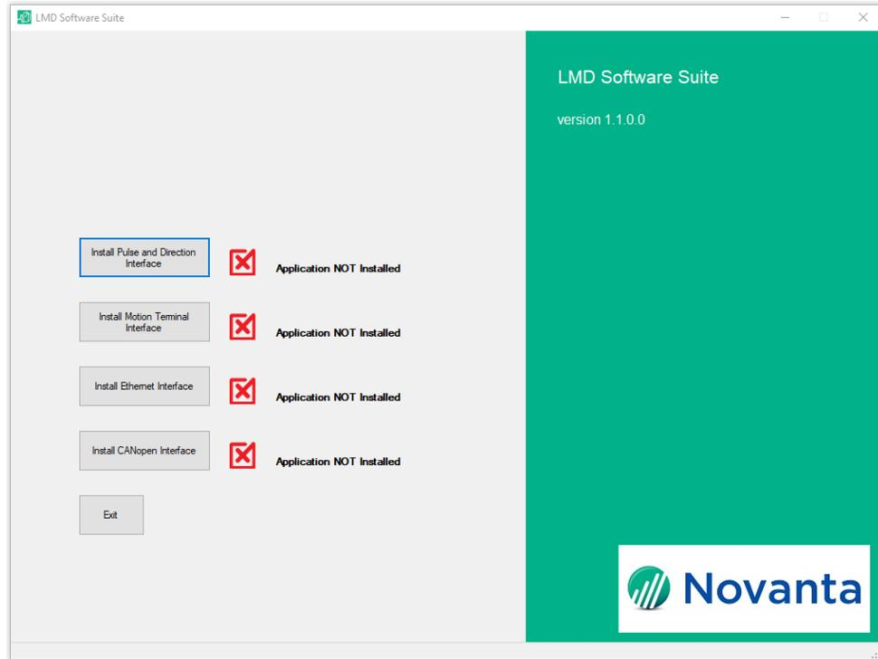
When first launched, a popup will be displayed indicating that no interfaces are currently installed and asking if all interface utilities should be installed. This is optional to the user. To install all interfaces, select Yes. To install a specific application, click No and select the application on the main screen that is appropriate to the device being used and follow the prompts for installation. Not all applications need to be installed.
