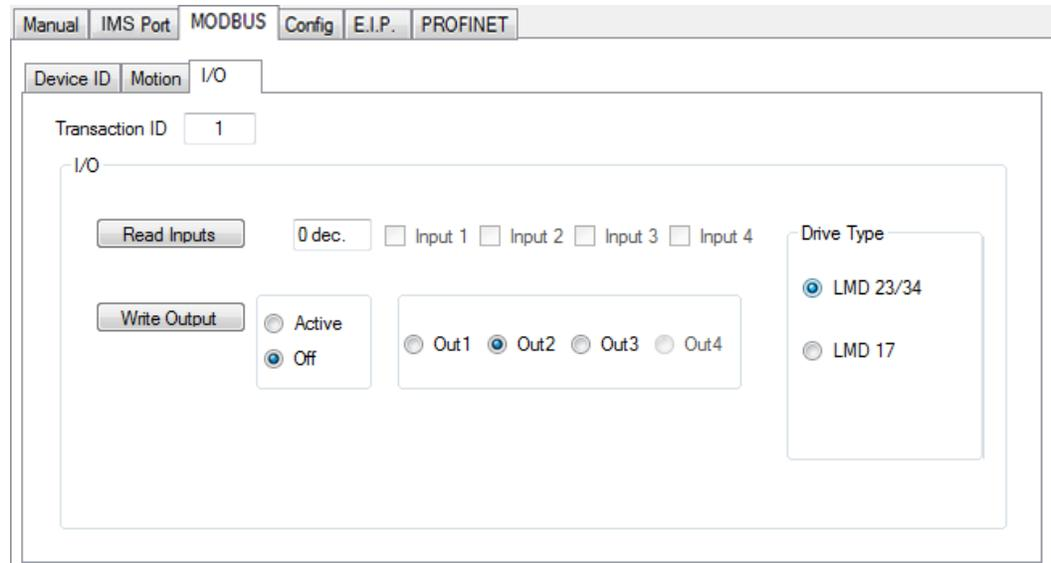
To test an I/O point, Click “Read Inputs”. The binary-coded-decimal state of the inputs will be read to the text field, The active inputs will be checked.
