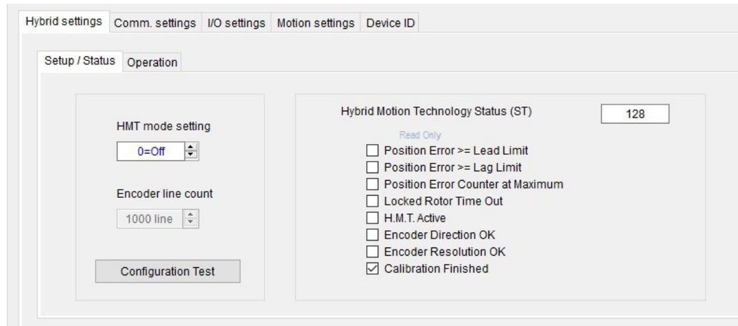
**NOTE:** hMT is only available on LMD Pulse/direction units with an internal encoder. These tabs will not be visible on units without an encoder.
