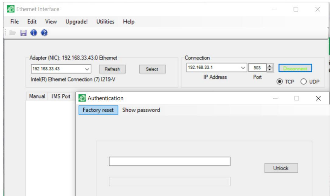
3. A message will be displayed providing information about the reset process. Click the “Agree “ check space and click “Return. The Factory password and IP Configuration reset dialog box will be displayed.
