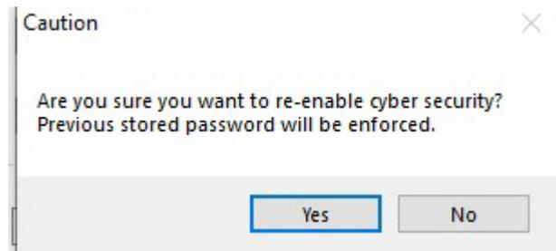
2. Click Yes to proceed with the re-enable of the cyber security password. The password will be re-enabled and set to the previously established password used prior to the disable.
