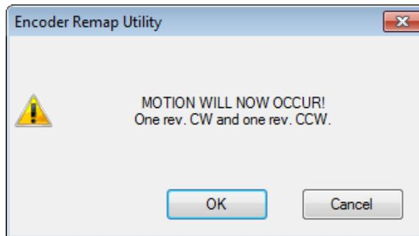
The motor will turn one revolution clockwise, then one revolution counter-clockwise. The device has been successfully remapped.
