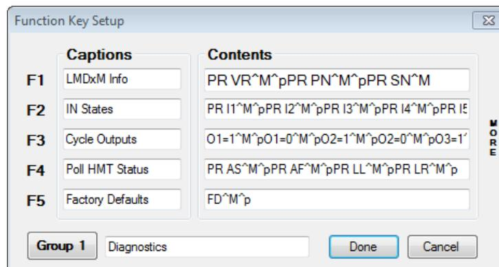
As shown above, function keys are defined by a string of MCode commands and control codes.
