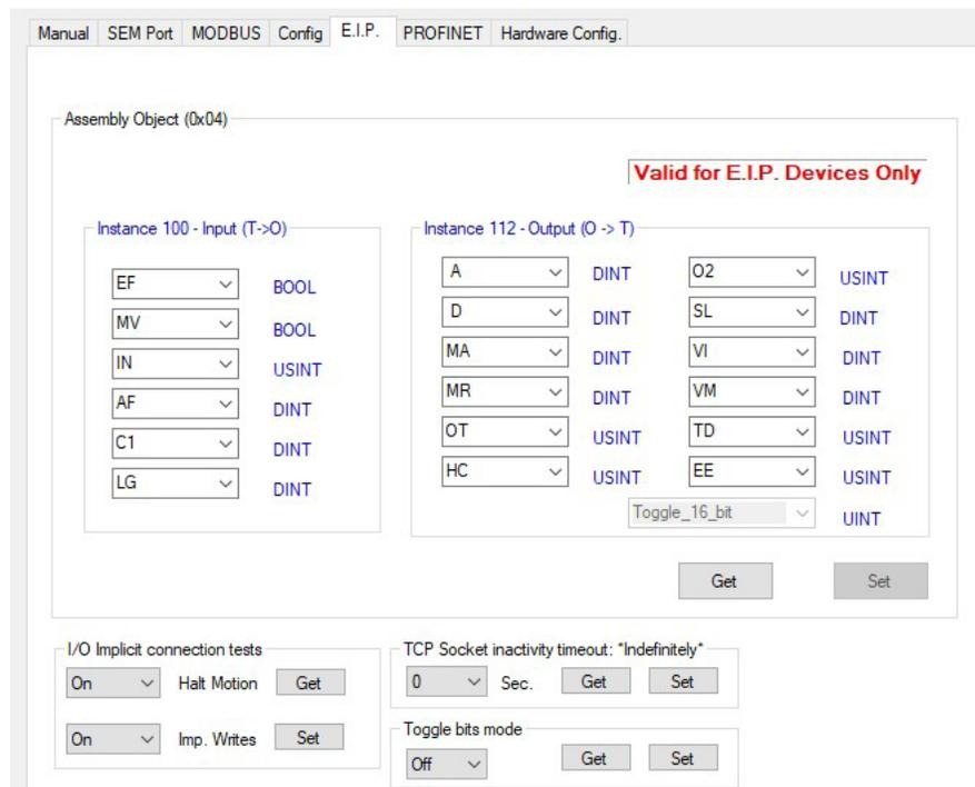
The EtherNet/IP configuration options contained in the TCP/IP Configuration Utility is variable mapping of the EIP assembly object.
