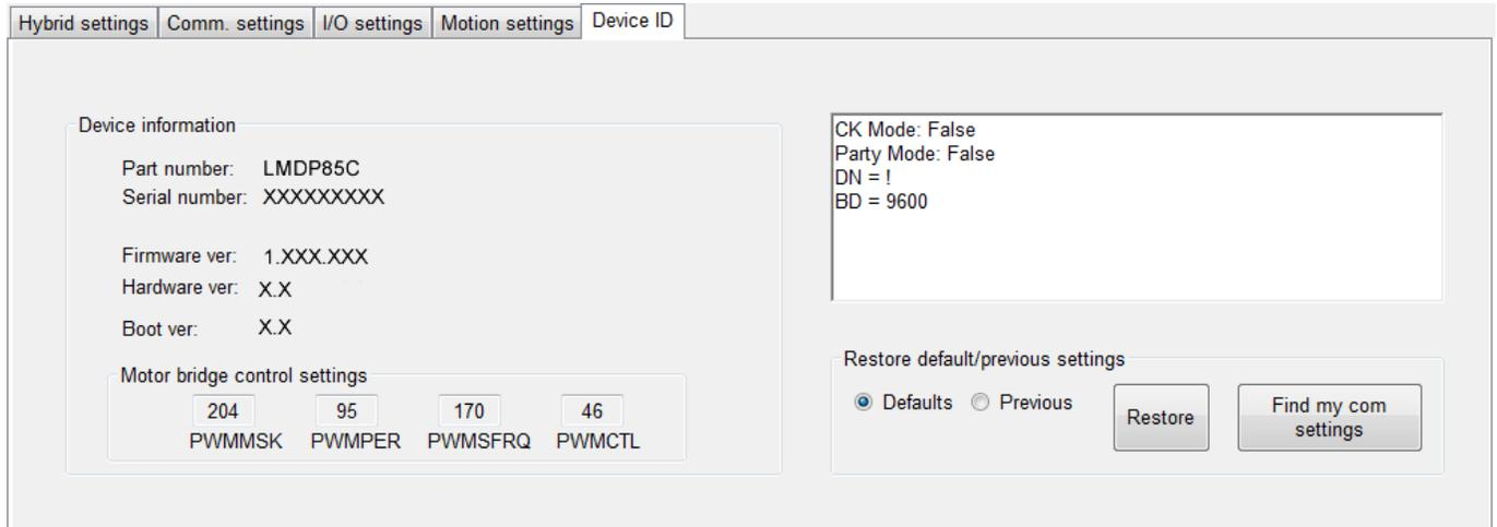
The Device ID tab contains the relevant information such as part number, serial number, and firmware and hardware versions.
