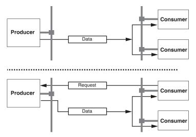
The producer sends a message that can be received by one or more network devices. The producer does not receive an acknowledgement to the effect that the message was received. The message transmission can be triggered by:
