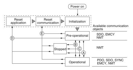
In the figure above, the communication objects available for use in the specific network state are shown on the right.
