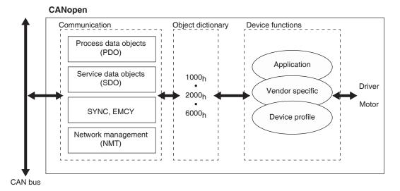
The object dictionary contains objects for describing the data types and executing the communication tasks and device functions under CANopen.
