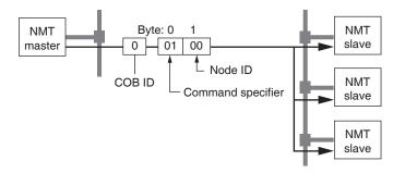
The first byte, the "Command specifier", indicates the NMT service used.
