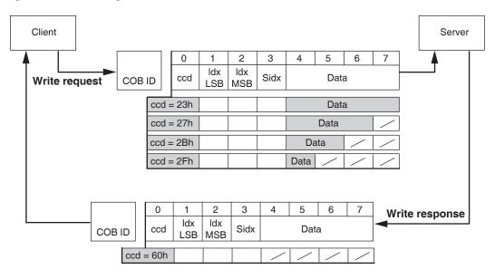
Unused bytes in the data field are shown with a slash in the graphic. The content of these data fields is not defined.
