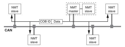
The LMD and LMD devices can only take on the function of an NMT slave.
