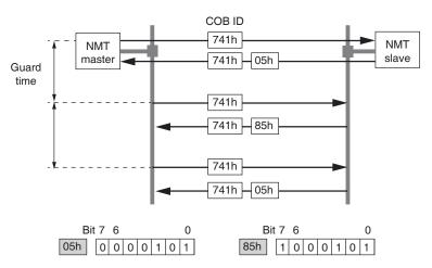
Bits 0 to 6 identify the NMT state of the slave:
