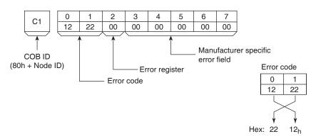
Bytes 0, 1 - Error code, value is also saved in the object Error code (603Fh) Byte 2 - Error register, value is also saved in the object Error register (1001h) Bytes 3, 4 - Reserved
