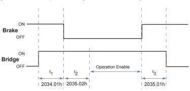
Figure B.13 - Output H-bridge to Brake Timing
