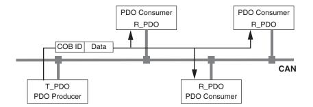
Data exchange with PDOs follows to the producer-consumer relationship and can be triggered in 3 ways:
