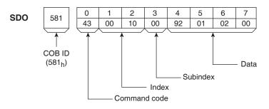
COB ID and data frame R\_SDO and T\_SDO have different COB IDs.
