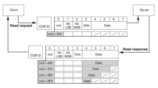
Figure 1.14 - Reading a Parameter Value
