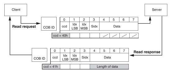
In the next frames, the remaining data is requested and transmitted in packets of 7 bytes from the server.
