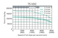
Test conditions: Load limits: maximum force/load is based on a static load. This will vary with a dynamic load.
