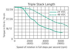
Test conditions: 100% current with damper simulating load.
