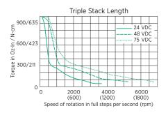
Test conditions: 100% current with damper simulating load.
