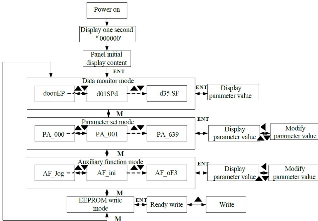
**Figure 7-2 the flow diagram of panel operation**
