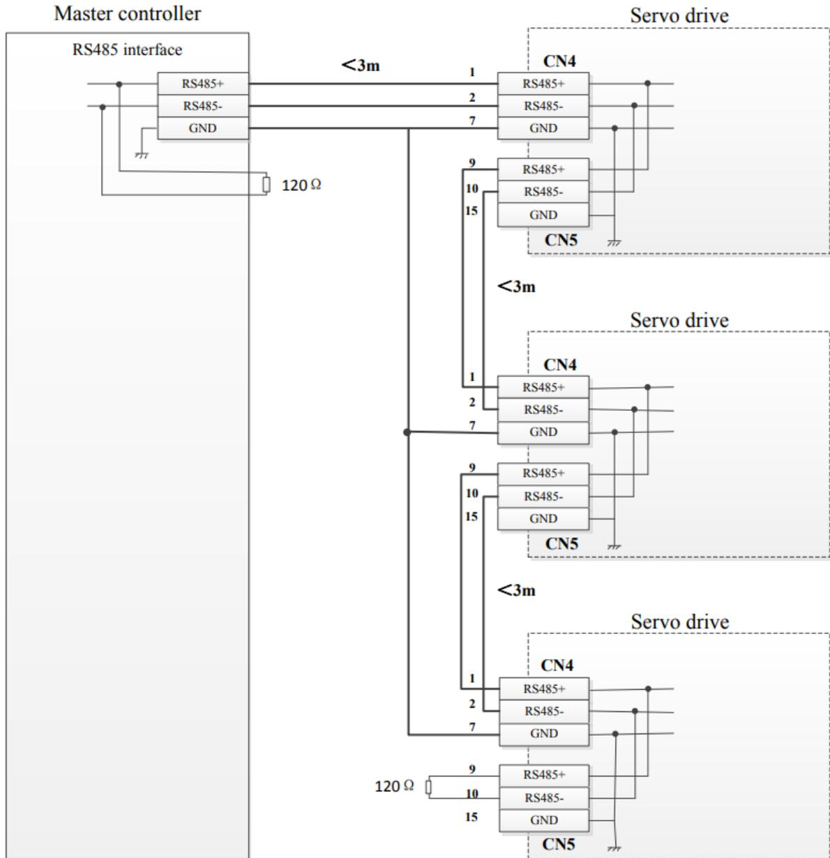
Figure: Multi-drive network connection
