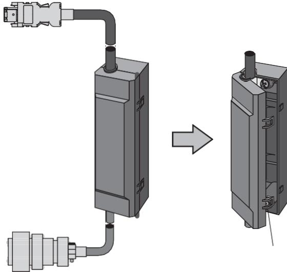
(3) Install the battery to the battery box.
