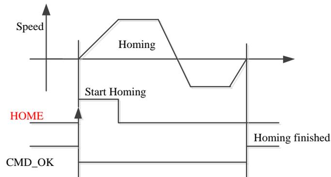
CMD\_OK and MC\_OK Both of them can be used to represent action is complete, after the signal effective, there will have a delay within 1 ms.
