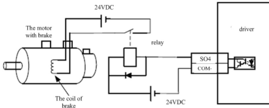
About the wire of brake, there should be an 24VDC for brake, the brake will be loosed with the 24VDC input, and the drive give an output signal to control the connection or disconnection of the 24VDC, pin 31 and pin 35 of CN1 is the control signal, and it is forbidden to connect these signal directly for the power of 24VDC, it will destroy the hardware of servo drive.
