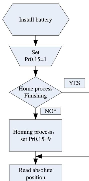
\*Note: The newly installed encoder is not initialized and will alarm
