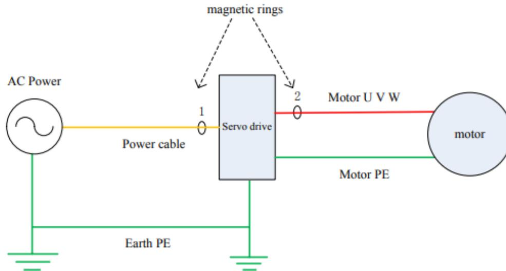
When there is an internal interference signal in communication, magnetic rings can be placed at 1 and 2 in above figure to suppress the incoming internal interference signal into the bus. Loop the UVW line around the magnetic ring three times. Be careful not to connect PE to the magnetic ring.
