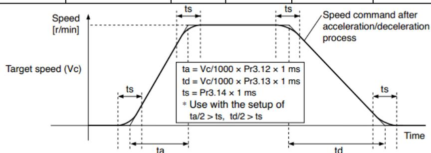
Set S-curve time for acceleration/deceleration process when the speed command is applied. According to Pr3.12 Acceleration time setup and Pr3.13 Deceleration time setup, set up sigmoid time with time width centering the inflection point of acceleration/deceleration.
