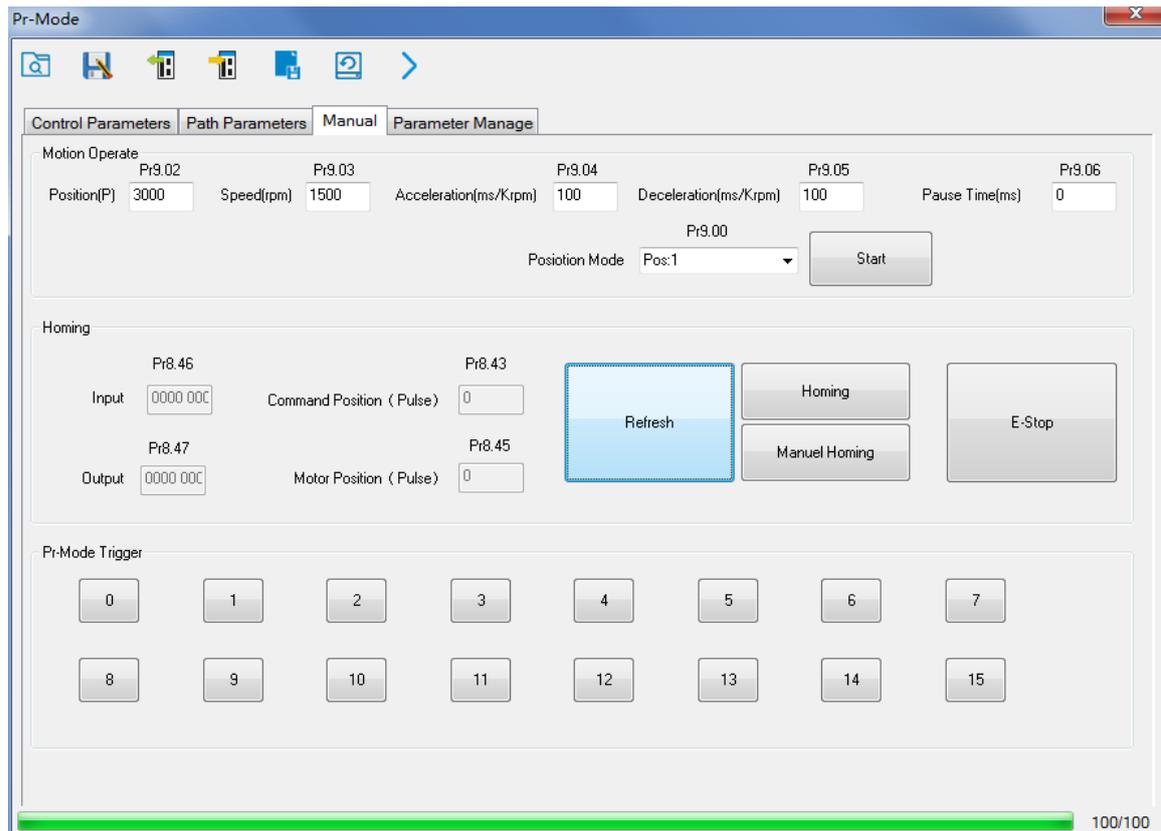
**Notes 1:** Before using IO CTRG edge signal trigger path motion, select path number by IO combined signal, and then use IO CTRG edge signal to trigger the corresponding path motion
