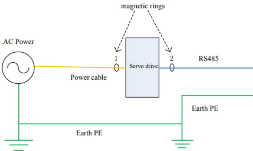
When there is an external interference signal in communication, magnetic rings can be placed at 1 and 2 in above figure to suppress the incoming external interference signal into the bus.
