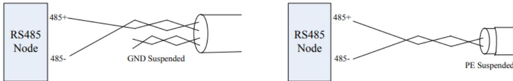
Firstly, confirm that the signal line of RS485 is connected correctly. Secondly, confirm whether the communication reference ground is connected correctly. If the node has no communication reference ground, it will be suspended, as shown in figure above. The shielding PE is connected the same way.
