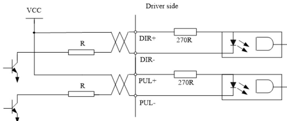
$V_{cc} = 12V, R = 1K, 0.25W; V_{cc} = 24V, R = 2K, 0.25W$
