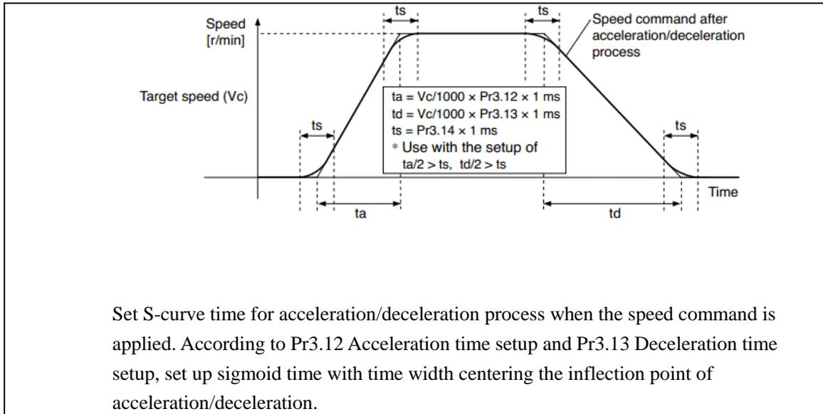
Set S-curve time for acceleration/deceleration process when the speed command is applied. According to Pr3.12 Acceleration time setup and Pr3.13 Deceleration time setup, set up sigmoid time with time width centering the inflection point of acceleration/deceleration.
