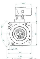
Power connector 4+4 PIN M23 turnable BEDC 110 - Signal connector 17 PIN M23 turnable AEDC 139
