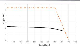
Continuous duty (S1) operation with cooling system appropriately sized.
