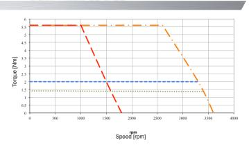
$\label{lem:continuous} \mbox{Continuous duty (S1) operation with cooling system appropriately sized.}$
