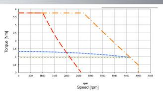
Continuous duty (S1) operation with cooling system appropriately sized.
