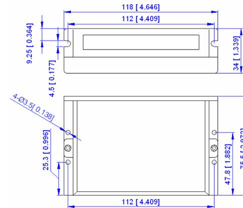
Figure 1: Mechanical specifications
